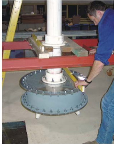
Figure 4 – Riser Cap Hydraulic Testing
