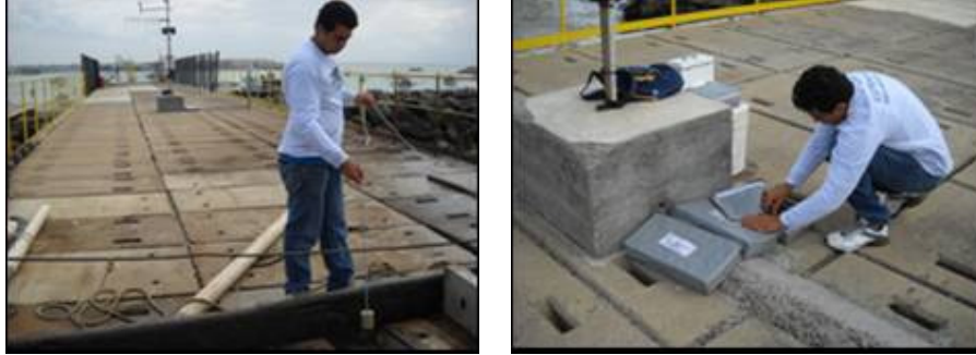
Figure 2. Sampling in a place where the dye tracer is completely mixed with effluent
