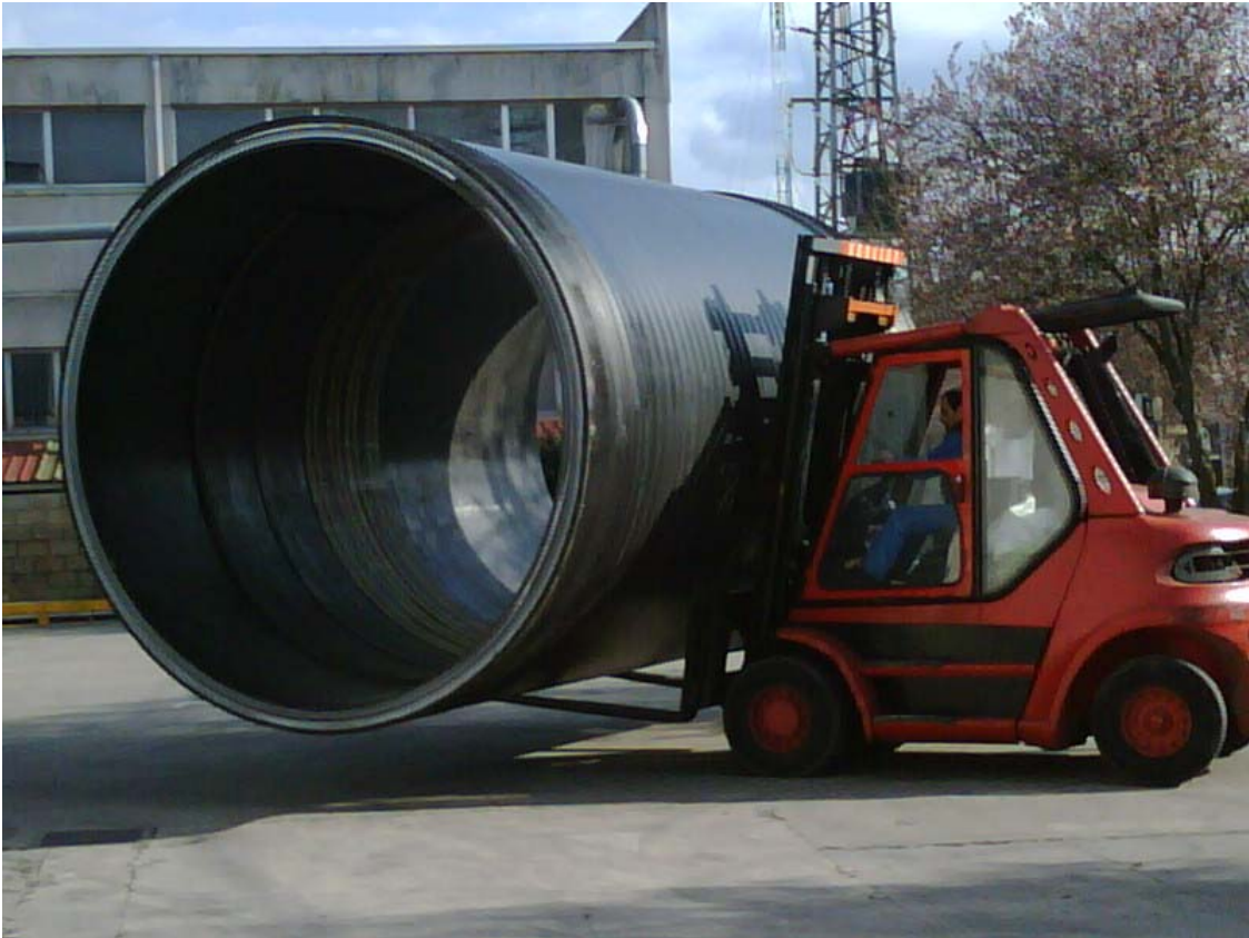
Figure 1 Pipe 3 m internal diameter for La Taboada
