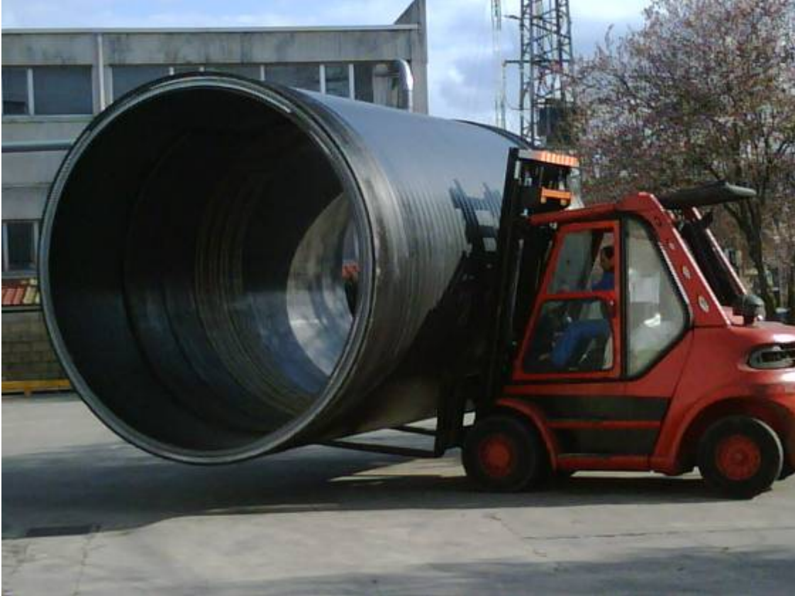
Figure 1 Pipe 3 m internal diameter for La Taboada
