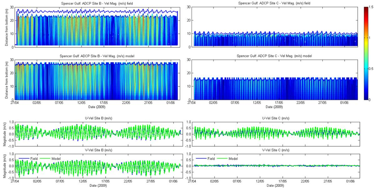
**Figure 2 Model Comparisons to Field Data at Sites B and C (see Figure 1). Upper Panels: Velocity Magnitude. Lower Panels: Depth-Averaged Velocity Components.**
