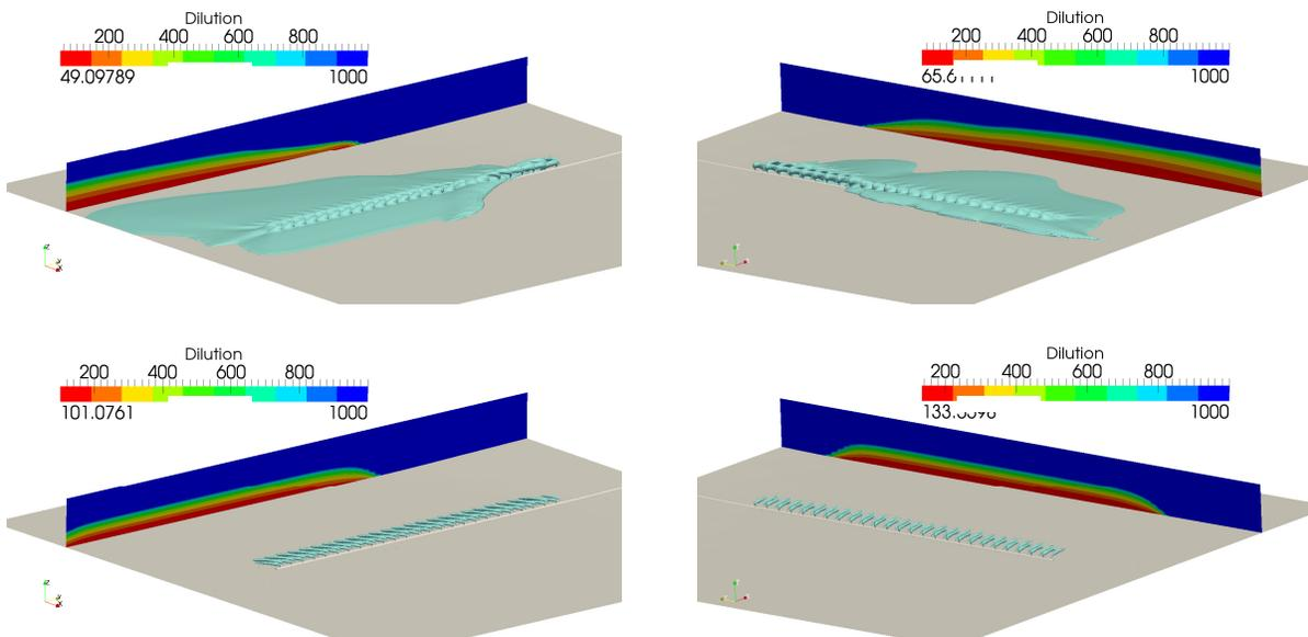
**Figure 3 Dilution Fields Obtained from the Nearfield CFD Simulations. Top Panels: Associated with 30<sup>th</sup> Percentile Velocity Profiles. Lower Panels: Associated with 70<sup>th</sup> Percentile Velocity Profiles. Left Panels: Ebb Tides. Right Panels: Flood Tides. See text for details.**
