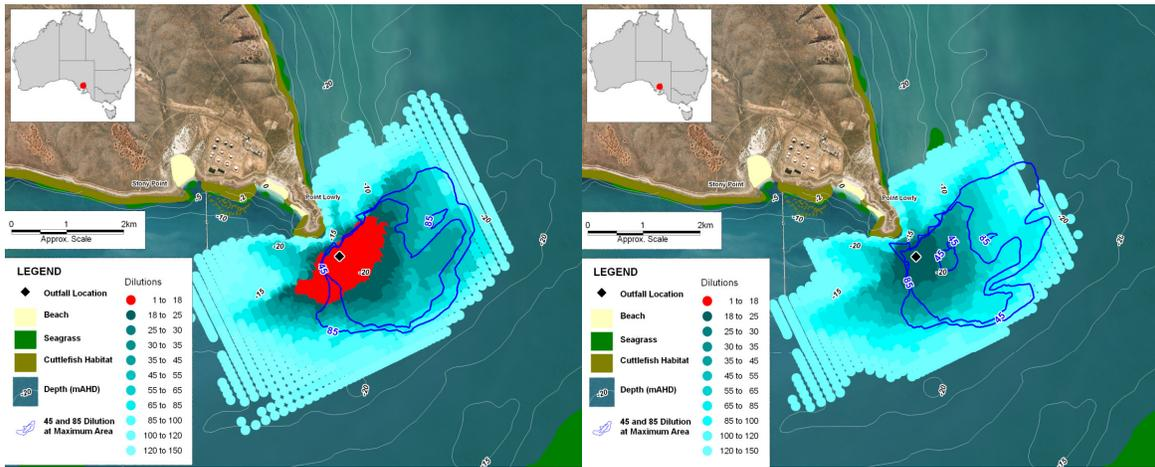
**Figure 7 Discharge Footprint given by 1<sup>st</sup> Percentile Dilution Maps. Left Panel: Direct Injection Method and Right Panel: Adaptive Injection Method.**
