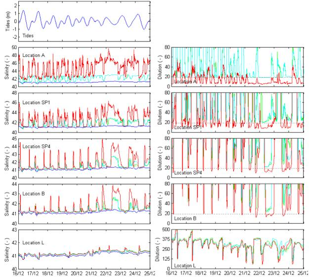
**Figure 6 Left Panel: Control Point Locations. Centre Panel: Salinities at Control Points. Right Panel: Dilutions at Control Points. Blue lines are background conditions, red lines are results of the direct insertion method, cyan lines are the adaptive linkage method using a 8s time step, and green lines are the adaptive linkage method using a 24s time step, the black dotted line is the minimum outfall dilutions.**
