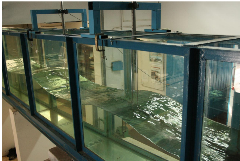
Figure 1: 23m Open Chanel in L.H. equipped of a wave generator with dynamic absorption
