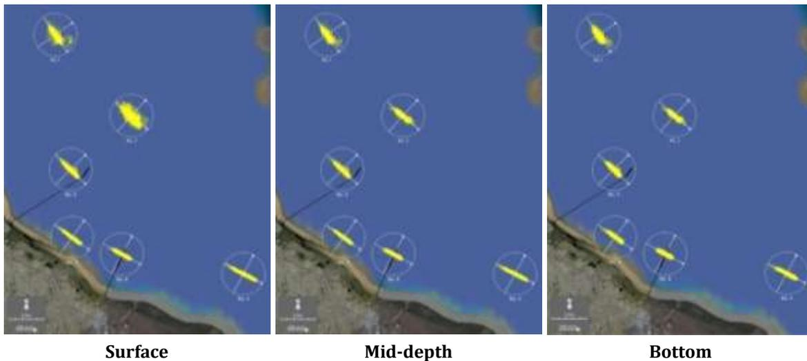
Figure 7. Polar scatter diagrams and principal axes of currents, 16 June – 16 Sept, 2009
