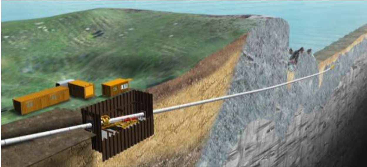
Picture 7 View of a Direct Pipe® construction site
