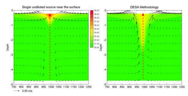
Figure 2 Comparison of flow fields (vertical cross section) in a schematic tank between the traditional, typical method of coupling (left) and the DESA coupling (right). The dashed red arrow shows the jet centreline that is schematised with the two different methods in the model.
