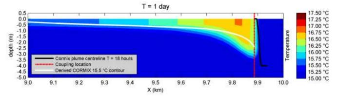
Figure 3 Preliminary results of a coupled CORMIX – Delft3D-FLOW computation. The contours in this vertical cross section along the plume show the temperatures derived by Delft3D-FLOW after coupling to CORMIX beyond the near field region (coupling location at red dashed line). The near field plume trajectory is presented in black. The Delft3D-FLOW results are compared to the CORMIX results in the derived 15.5°C contour line (white line).
