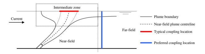
Figure 1 Typical plume behaviour including boundary interaction and lateral spreading along the water surface. The typical and preferred locations for coupling the near and far field are indicated.
