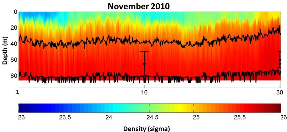
**Figure 5.** RSB model output illustrating predicted plume rise height and thickness based on plume density data input. Such outputs were generated before each mission to plan mission depth ranges. Observed mid-point, thickness, and rise height are shown for November 16<sup>th</sup> and 30<sup>th</sup> missions. The depth range chosen for each mission based on this output was 30 -90 m.
