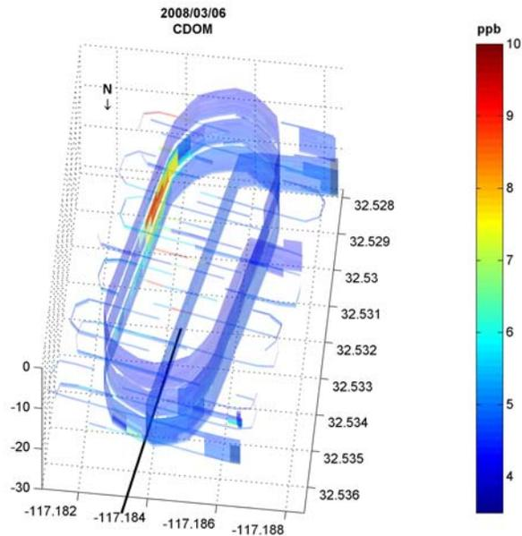
**Figure 8.** SBOO Plume Organic Matter Concentrations. Elevated values of CDOM (>7 ppb) indicate high concentrations of organic matter in the SBOO plume. The SBOO is shown in black with the observed plume toward the south-southeast. The observed plume is coincident with the plume trajectory (colored lines) estimated from the SBOO buoy velocity profiles.
