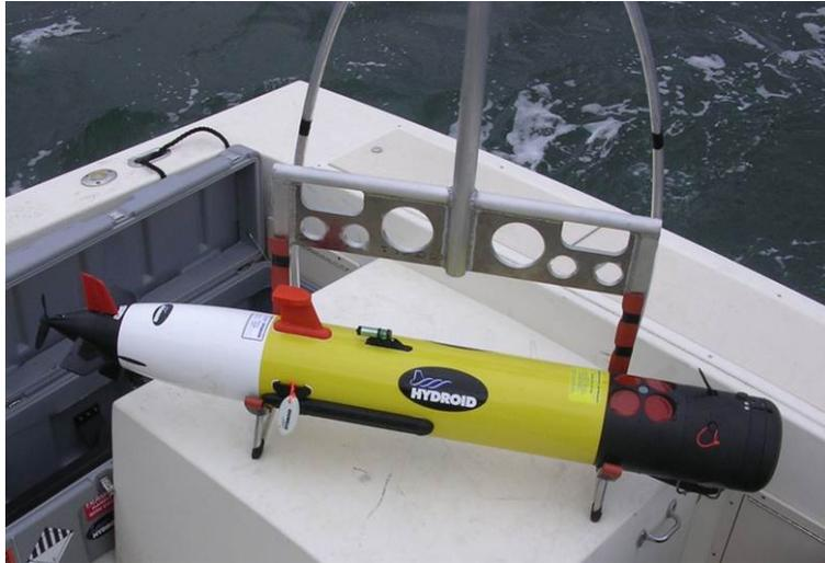
**Figure 3.** The Remote Environmental Measuring UnitS (REMUS) vehicle on board prior to deployment uses GPS, an acoustic doppler current profiler (ADCP), conductivity, temperature, depth (CTD), optical backscatter, and colored dissolved organic matter sensor (CDOM).
