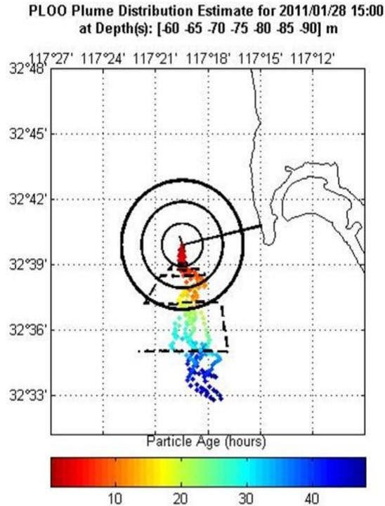
**Figure 6.** Near real-time PLOO plume trajectory estimate for depths of 60, 65, 70, 75, 80, 85, and 90 m from the PLOO mooring buoy. The 2D monitoring mission (dotted line) was designed to optimally sample the plume location within the constraints of the vehicle’s operating parameters. Circles at 1 km, 2 km, and 3 km radius give approximate distance from the outfall.
