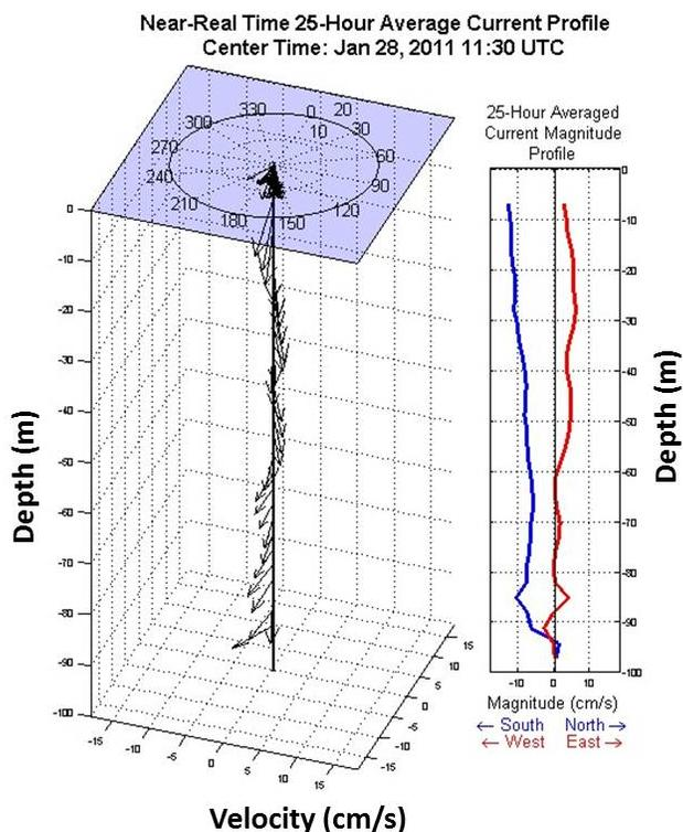
**Figure 7.** A 25-hour averaged ADCP profile plot for January 28, 2011 used to plan a PLOO monitoring missions. The profile shows a southerly current direction (blue line) with little east/west current in the bottom half of the water column (expected plume depths).
