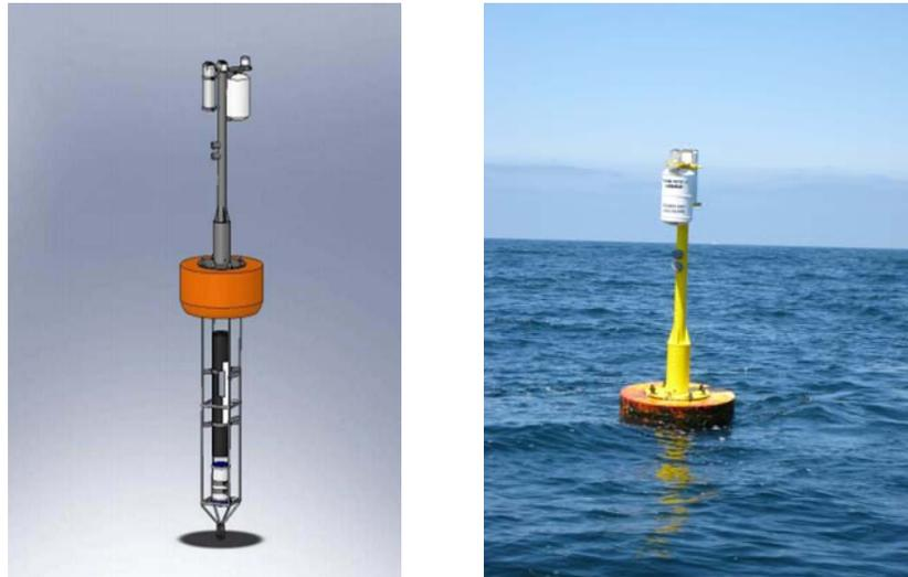
**Figure 2.** Drawing and a photograph of the Scripps-designed coastal buoy system for measuring stratification and currents at the South Bay and Point Loma Ocean Outfalls.
