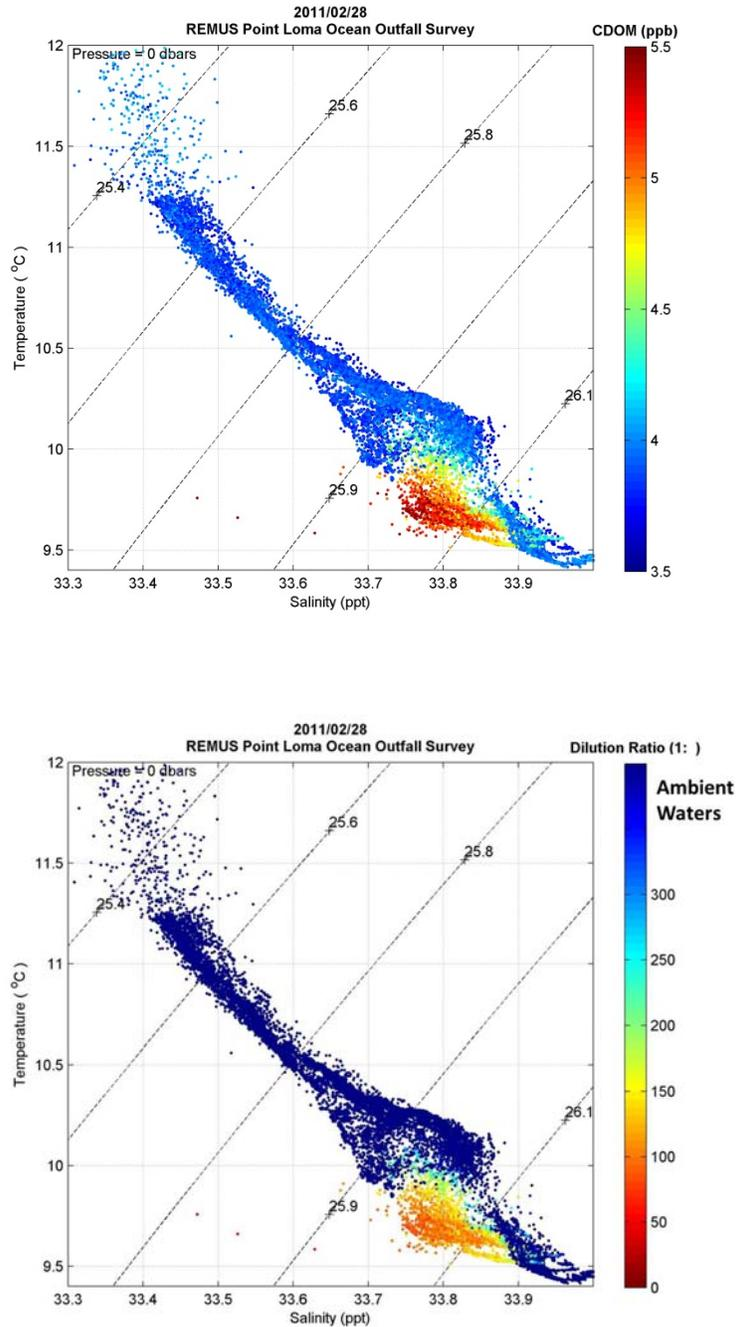
**Figure 11.** A CDOM T-S diagram (top) for the February 28<sup>th</sup>, 2011 PLOO mission. The CDOM signature of the plume clearly separates it from surrounding ambient water. These data are used to calculate the dilution field seen in the bottom plot. According to the plot, the core of the plume has dilutions around 1:100.
