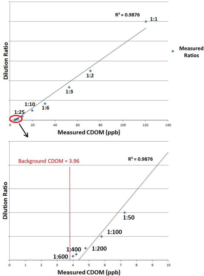
**Figure 10.** A CDOM calibration curve of source effluent from the Point Loma Wastewater Facility. The effluent was mixed with seawater (background CDOM = 3.96) to create a range of dilutions from 1:1 to 1:600. The WETlabs ECO triplet used on the REMUS was used to measure CDOM concentrations at each dilution ratio. The graph shows a linear trend with successful measurement of CDOM signatures up to a dilution of 1:600 before background contamination.
