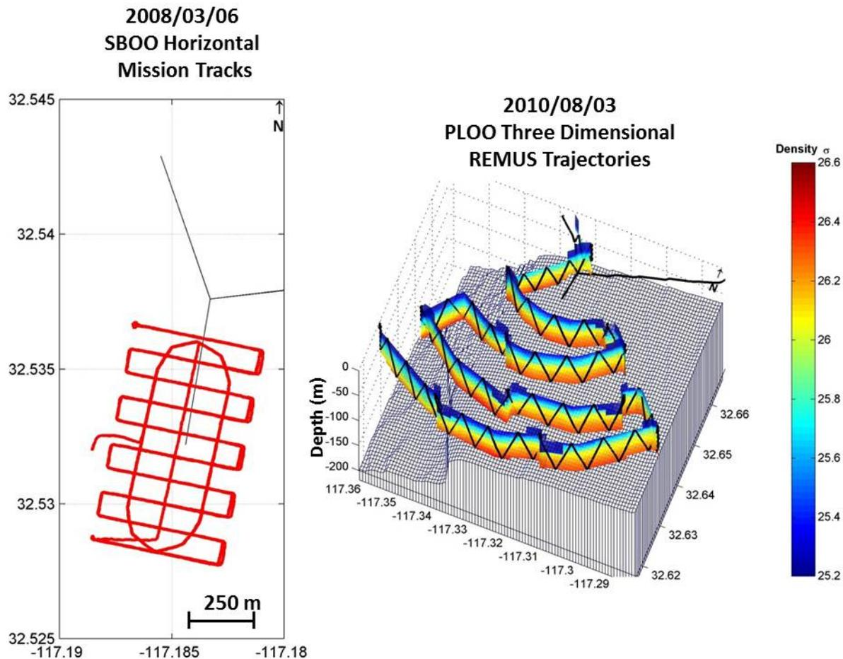
**Figure 4.** Examples of 2D SBOO and 3D PLOO mission tracks for March 6<sup>th</sup>, 2008 and August 3<sup>rd</sup>, 2010 respectively. a) *SBOO*: The lawnmower-like pattern was measured at approximately 20 m, 15 m, and 10 m while the oval was measured using 6 m saw tooth pattern for depth ranges 3 – 9 m, 10 – 16 m, and 17 – 23 m. b) *PLOO*: Saw tooth trajectory pattern typical for far-field missions. Horizontal resolution between saw tooth measurements is approximately 450 m.
