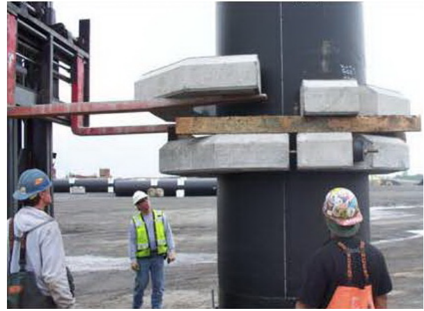
Figure F – Testing the sliding resistance of a collar. Notice the gap between the two halves of the secured collar.
