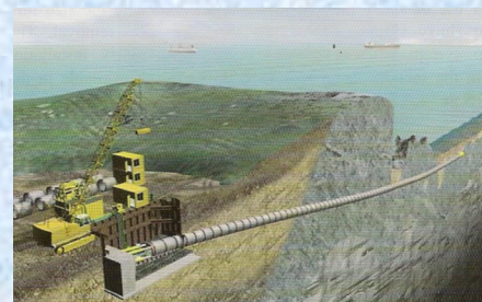
Schematic of a jacked outfall from a cliff top (Courtesy Herrenknecht AG)
